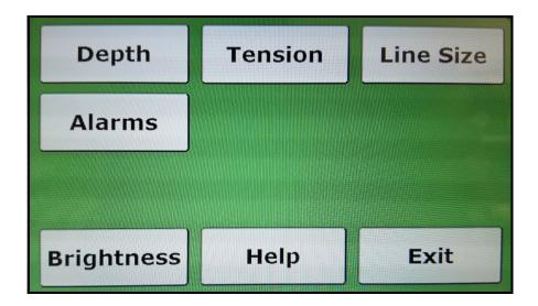
In this Menu you can select any of the above settings to change. Brightness will toggle the panel to a higher brightness mode for sunlight readability. The Help menu is available in both the Left and Right Menus.
