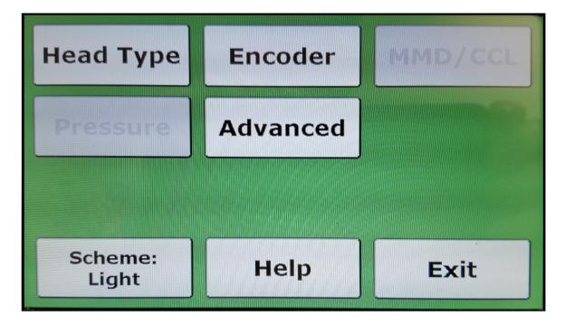
**2.1.5 Select Encoder parameters**. You can set parameters for 1 encoder, 2 separate encoders or set both at the same time.
