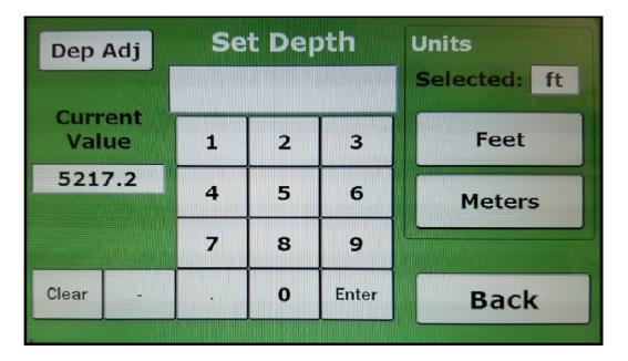
This menu is where the Operator can set the system depth.
