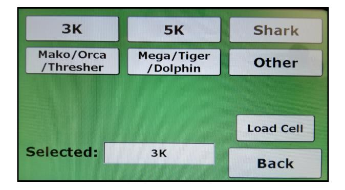
This panel is capable of both Wireline and Slickline, requiring the operator to select the measuring head the system will be reading.
