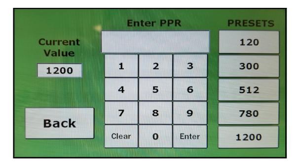
This menu is to set the Encoder Pulse rate to match the Encoder on the measuring head. The operator can select from a list of common BenchMark pulse rates on the right, or enter a new value manually.
