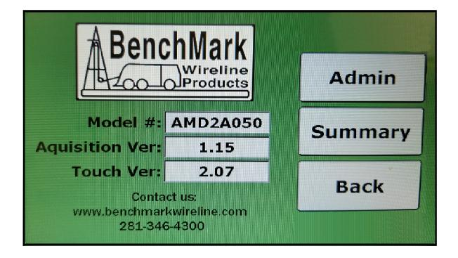
The help menu allows the operator to see the model number, software versions for troubleshooting, and contact information for BenchMark Wireline Products. It also contains the buttons to get to Admin controls and Summary.
