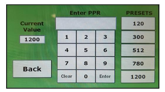
**2.1.7 PPF - If you are using an acquisition system like Warrior**, you would additionally set Encoder Output Pulses to allow the panel and the acquisition systems to sync with each other.
