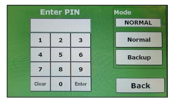
The Admin menu is a new feature introduced in this panel. It allows the operator to get to the Backup Mode Select, but also allows the Supervisor to have additional control over the panel which was not available in previous versions. The default PIN is 00000 and can be set to a custom value once inside the ADMIN system.
