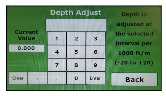
This is a Depth shim setting that can be used to correct for wheel wear compared to a known depth. It is selected from the above Depth Menu.
