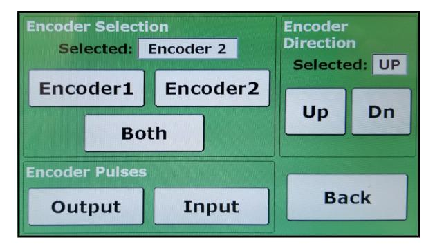
**2.1.6** PPR - Then select Input for input pulse settings. The default is 1200 ppr or pulses per revolution on the head.
