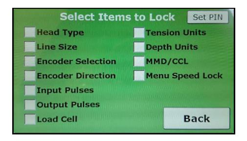
The Administrator controls are very simple, and allow the Supervisor to block the operator from changing settings in the list above. It also contains a lock which will not allow the panel to go into the Menu when the line is moving. It requires the operator to stop before making any adjustments.
