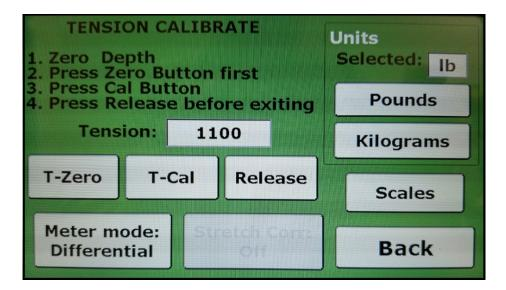
The Tension menu is where the Operator can Calibrate Tension, select the left meter setting between differential and incremental tension, set units, enable/disable stretch correction, and set the scale values for both meters.
