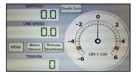
Both Displays are capable of running independently as shown. This allows the operator to continue work in the event of a damaged display or error. This mode allows the operator to see Depth, Tension, Line Speed, and Differential tension all on one screen.
