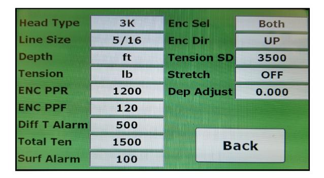
This is a quick way to see all current settings in the panel, and can be accessed via the HELP menu which is available on both displays.
