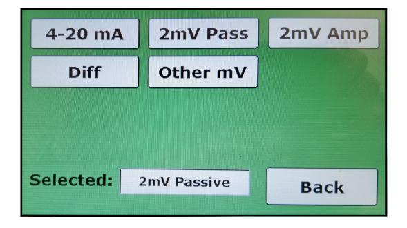
This panel also allows for many different Load Cell types and can be changed in this menu. An option to have 2 different load cells will be available in the future.
