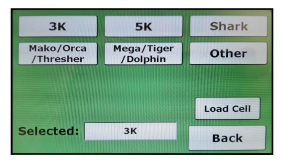
**2.1.3 Press the Load Cell button** and select the load cell type and press the **Back** button 2 times.
