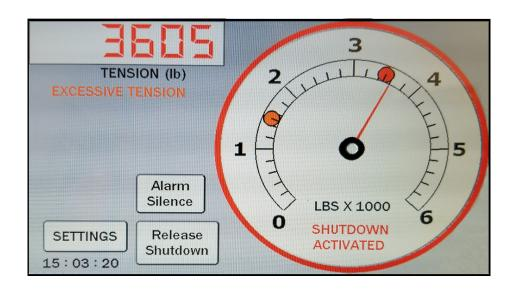
Tension – The panel is capable of displaying Total Tension, Differential Tension and Incremental Tension
