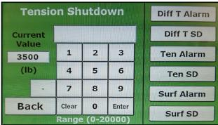
These four menus are selected by pressing the correlating menu button on the right hand side. The operator sets these values and the Dynamic Display alerts are automatically adjusted.
