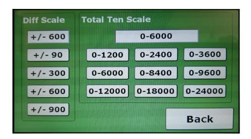
This menu is selected via the Tension menu and is used to set the scales displayed on both Meters.
