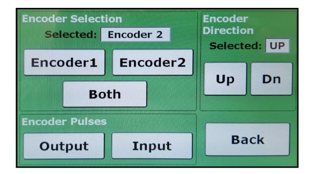
This menu allows the operator to select between encoders, and select depth units, as well as set the Optical Encoder incoming and outgoing pulse rates.
