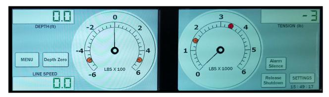
The above configuration is the default display of the AMD2A040. The display contains Depth, Tension and Line Speed, as well as current time in the lower right corner. The left screen contains the differential tension meter which can be set in either Differential or Incremental mode. The yellow dots indicate differential tension alarm settings. The Depth Zero button will set depth to 0, but can be pressed again to see the previous depth.
